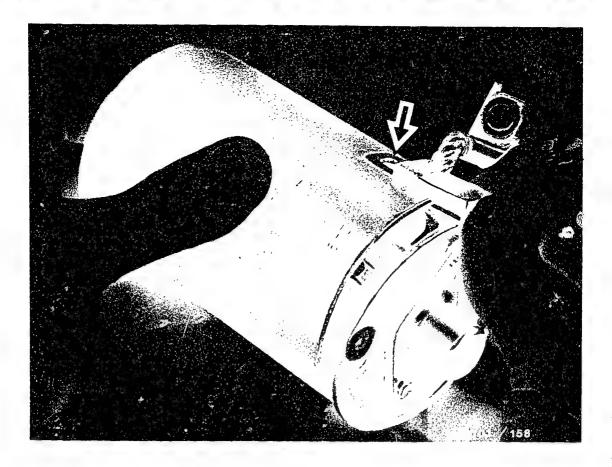
11.4 Assembling the stator frame (DW starting motors)
